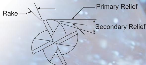
**Primary Relief** – The clearance directly behind the cutting edge. High primary relief angles will allow for more aggressive milling, while lower relief angles will increase the strength of the cutting edge. The primary relief will also affect the wear on a cutting edge. Lower primary relief angles can tend to develop larger wear lands.
