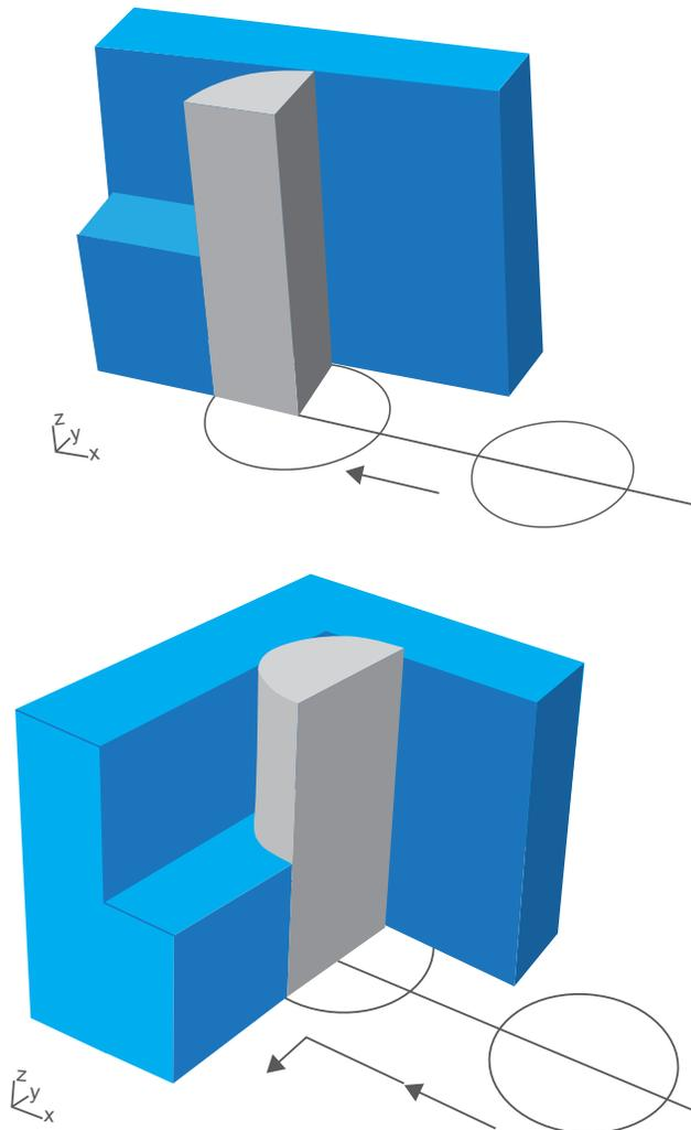
At this intersection, large engagement would cause tool chatter and even breakage. Using CAD CAM software to generate the corner avoids an abrupt stop and change of direction. It also keeps a constant arc of engagement while providing smooth chatter free cutting and long tool life.
