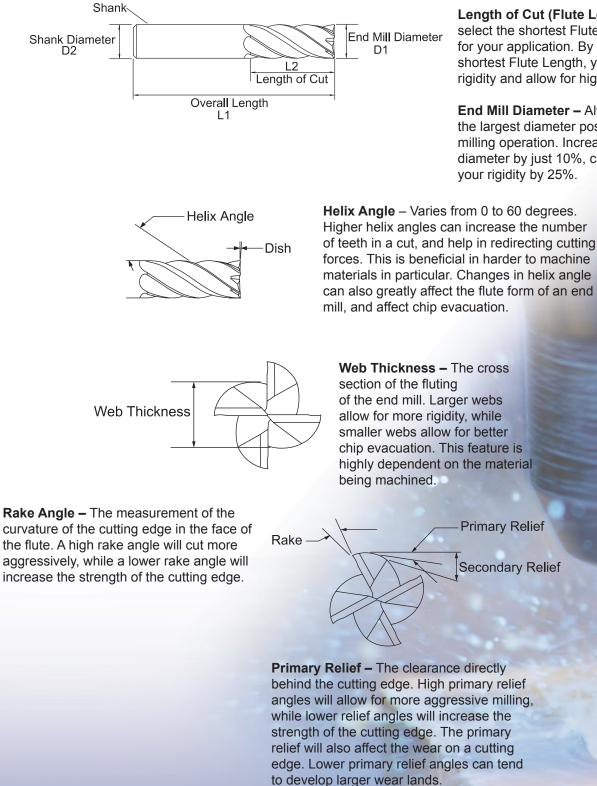
Length of Cut (Flute Length) – Always select the shortest Flute Length possible for your application. By selecting the shortest Flute Length, you can increase rigidity and allow for higher feed rates.
